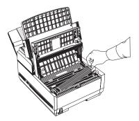
9. Once the toner cartridge is in place, push the colored lever all the way forward to secure it and release the toner.
